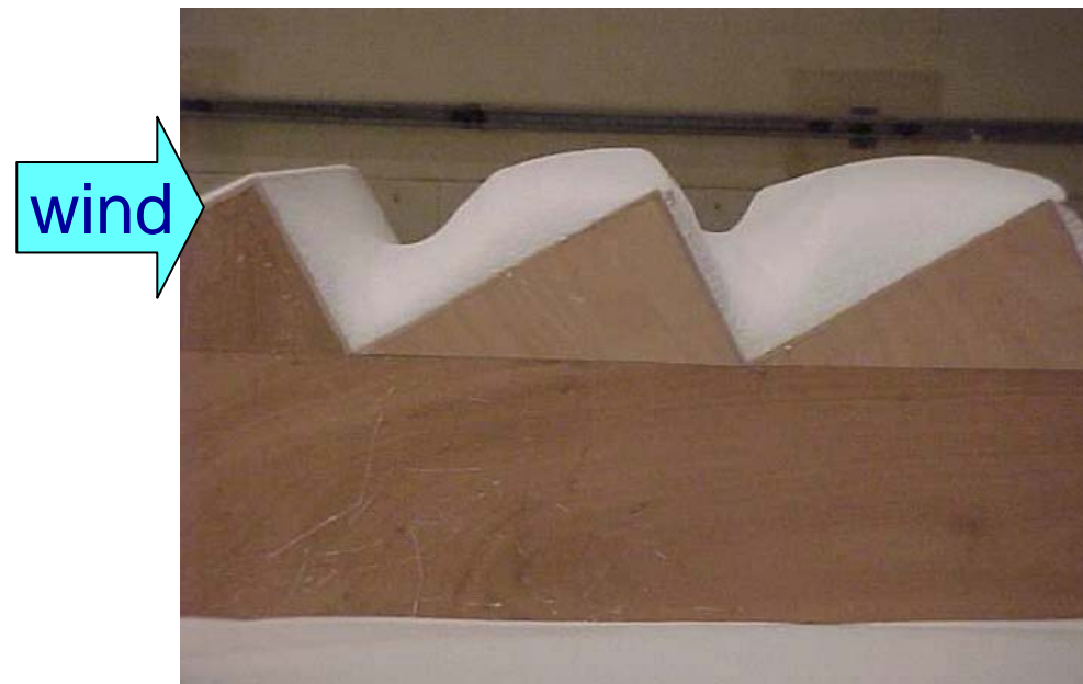
Model in wind tunnel for multi - pitched roof wind velocity > 5 m/s
