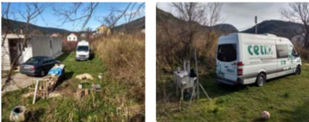
Figures 9-10. Mobile unit and sequential sampling device for particulate matter in the ambient air (measuring point 3)
