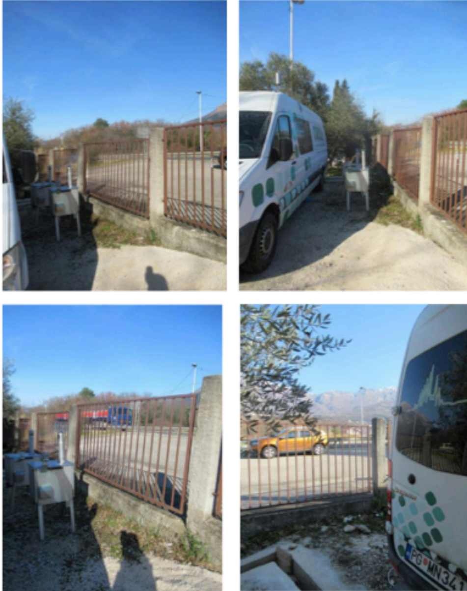
Figures 1-4. Mobile unit and sequential sampling device for particulate matter in the ambient air (measuring point 1)
