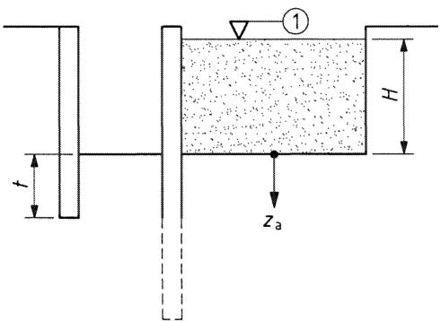
b) Where the piezometric surface and the **ground-water tables** are **above the excavation base**, the larger value of the following conditions should be met:
