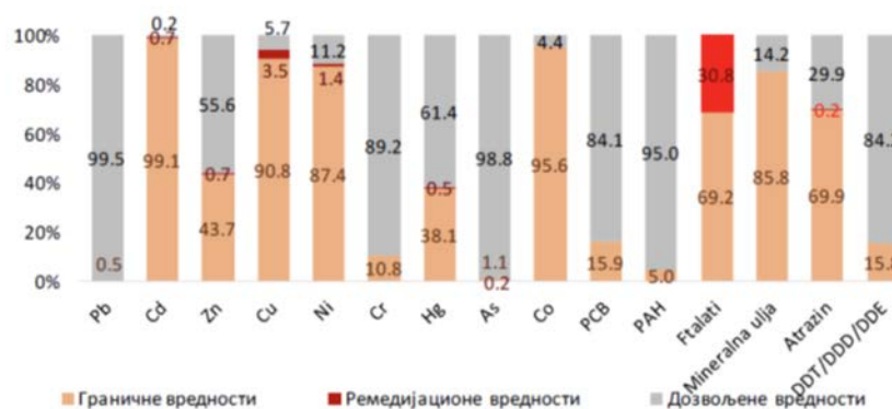
Figure 1.32. The exceedance percentages at the depth of 30-60 cm, at landfill central points (AP Vojvodina)
