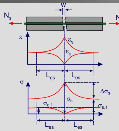
Change of stresses in reinforcement due to cracking:
