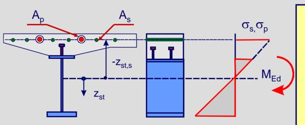
Stresses  $\sigma_s^*$  in reinforcement at the crack location neglecting different bond behaviour of reinforcement and tendons:
