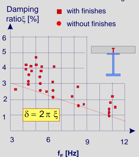
For the determination of the maximum acceleration the damping coefficient  $\zeta$  or the logarithmic damping decrement  $\delta$  must be determined. Values for composite beams are given in the literature. The logarithmic damping decrement is a function of the used materials, the damping of joints and bearings or support conditions and the natural frequency.
