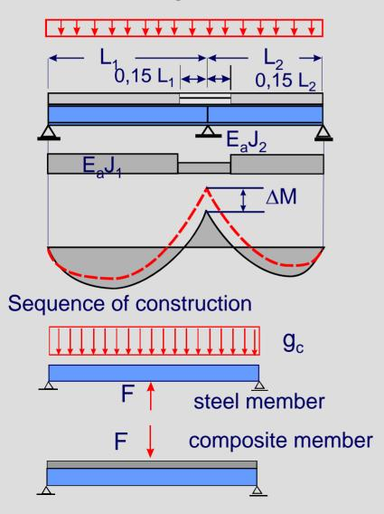
Deflections due to loading applied to the composite member should be calculated using elastic analysis taking into account effects from
