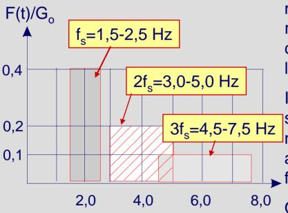
People in office buildings sitting or standing many hours are very sensitive to building vibrations. Therefore the effects of the second and third harmonic of dynamic load-time function should be considered, especially for structure with small mass and damping. In case of walking the pacing rate is in the rage of 1.7 to 2.4 Hz. The verification can be performed by frequency tuning or by limiting the maximum acceleration.
