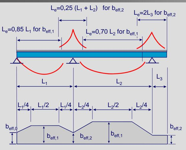
end supports:  $b_{eff} = b_0 + \beta_1 b_{e,1} + \beta_2 b_{e,2}$  $\beta_i = (0.55 + 0.025 L_e/b_i) \le 1.0$
