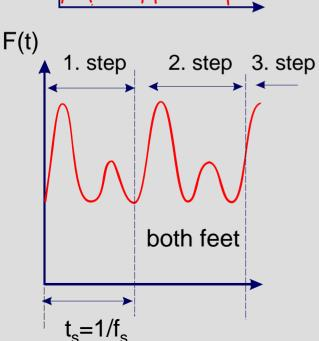
During walking, one of the feet is always in contact with the ground. The load-time function can be described by a Fourier series taking into account the 1st, 2nd and 3rd harmonic.
