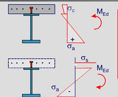
Stress limitation is not required for beams if in the ultimate limit state,
