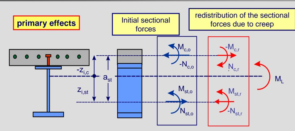
The effects of shrinkage and creep of concrete and non-uniform changes of temperature result in internal forces in cross sections, and curvatures and longitudinal strains in members; the effects that occur in statically determinate structures, and in statically indeterminate structures when compatibility of the deformations is not considered, shall be classified as primary effects.
