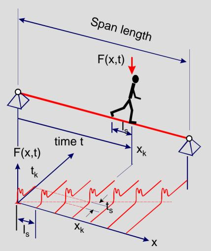
The pacing rate  $f_s$  dominates the dynamic effects and the resulting dynamic loads. The speed of pedestrian propagation  $v_s$  is a function of the pacing rate  $f_s$  and the stride length  $I_s$ .
