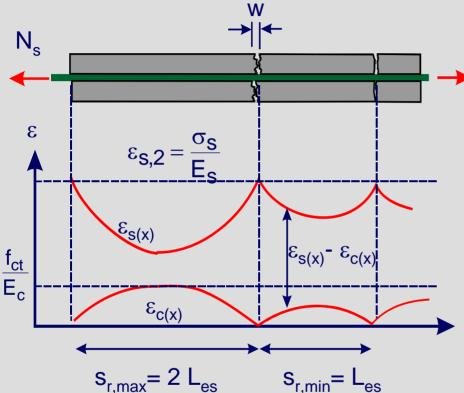
The maximum crack spacing  $s_{r,max}$  in the stage of stabilised crack formation is twice the introduction length  $L_{es}$ .
