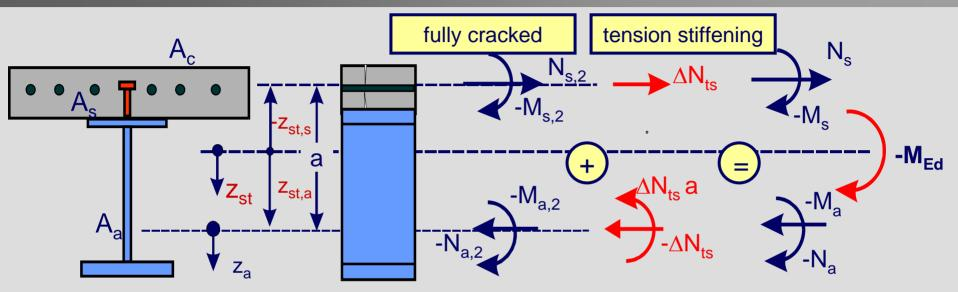
The calculation of stresses is based on the mean strain in the concrete slab. The factor  $\beta$  results from the mean value of crack spacing. With  $s_{rm} \approx 2/3$   $s_{r,max}$  results  $\beta \approx 2/3 \cdot 0.6 = 0.4$
