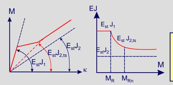
uncracked section fully cracked section E<sub>st</sub>J<sub>2.ts</sub> effective flexural stiffness taking into account tension stiffening of concrete
