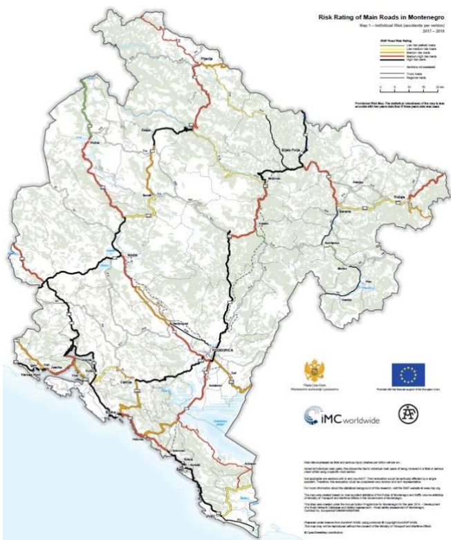
Figure 3.2. Road accident risk map per km Montenegro according to the iRAP methodology according to the iRAP methodology
