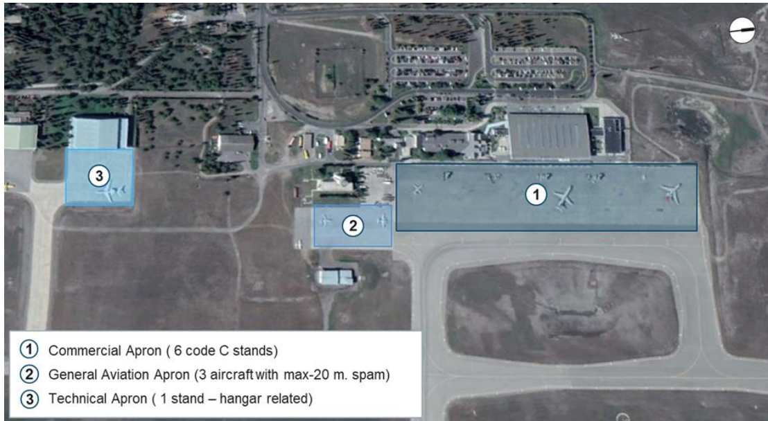
Figure 40 TGD Apron Configuration
