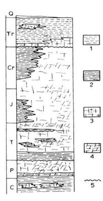
Fig. 21 Schematic lithostratigraphic column of Dinaric region (Herak, 1972). Legend: 1 = Tertiary clastic deposits; 2 = Palaeozoic and Mesozoic clastics; 3 = limestones; 4 = dolomites; 5 = main unconformities; C = Carboniferous; P = Permian; T = Triassic; J = Jurassic; Cr = Cretaceous; Tr = Tertiary; Q = Quaternary.
