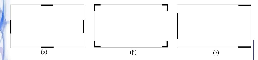
Arrangements of shear walls in plan:
