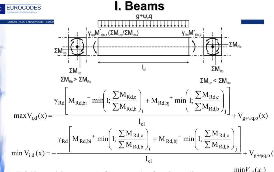
• in DC H  $\gamma_{Rd}$ =1.2 - reversal of V accounted for, depending on:  $\zeta_i = \frac{\min V_{i,d}(x_i)}{\max V_{i,d}(x_i)}$ in DC M  $\gamma_{Rd}$ =1.0,
