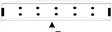
In-plane bending of long floor diaphragms in building with two strong walls at the 2 ends  $\rightarrow$  intermediate columns overloaded, compared to results of design w/ rigid diaphragm
