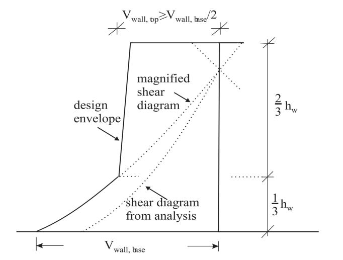
To account for increase in upper storey shears due to higher mode inelastic response (after plastic hinging at the base)
