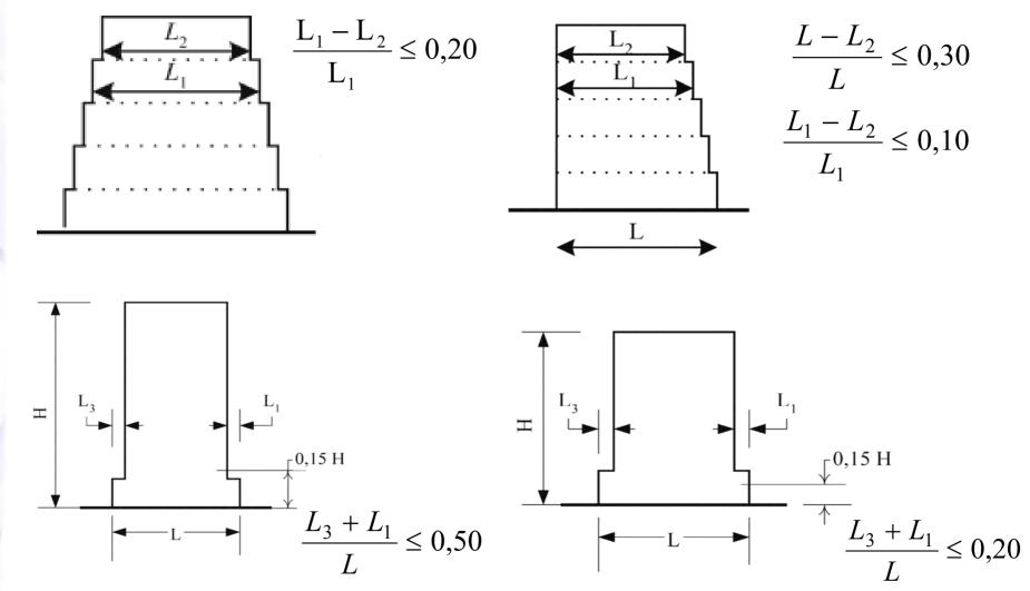
Eurocode 8 criteria for regularity in elevation in buildings w/ setbacks
